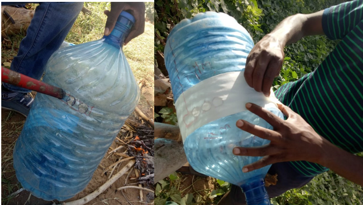
Figure 2a. Perforating a bottle with a hot metallic rod (Left); b) Strapping polyester textile around a bottle (right).
