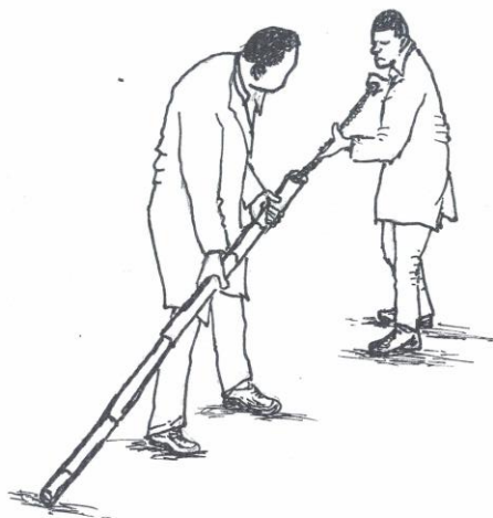
Figure 2: Punching the diaphragm using a long metal rod
