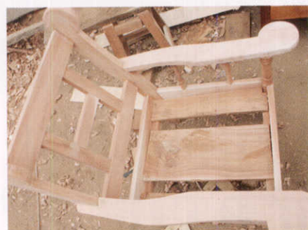
Detail of chair, manufactured from mukau wood in a rural workshop. Timber quality is deficient as almost all good trees have disappeared and small diameter logs with various defects are now being sourced.
