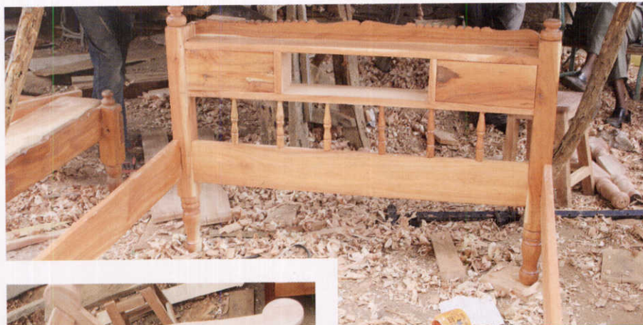
A bed frame made of mukau wood in a rural furniture workshop (Nuu, in Mwingi East). Mukau is highly valued for the quality of its timber, for various reasons including its resistance to termites. (Photo BGF)
