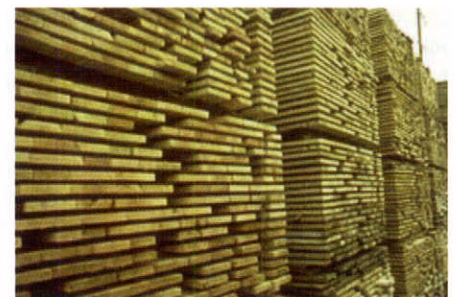
Photo 3: Inspection paths between timber stacks.
