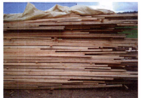
Photo 2: Poorly stacked timber.
