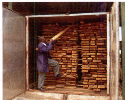
Photo 4: Stacking a kiln timber dryer at KEFRI Karura.
