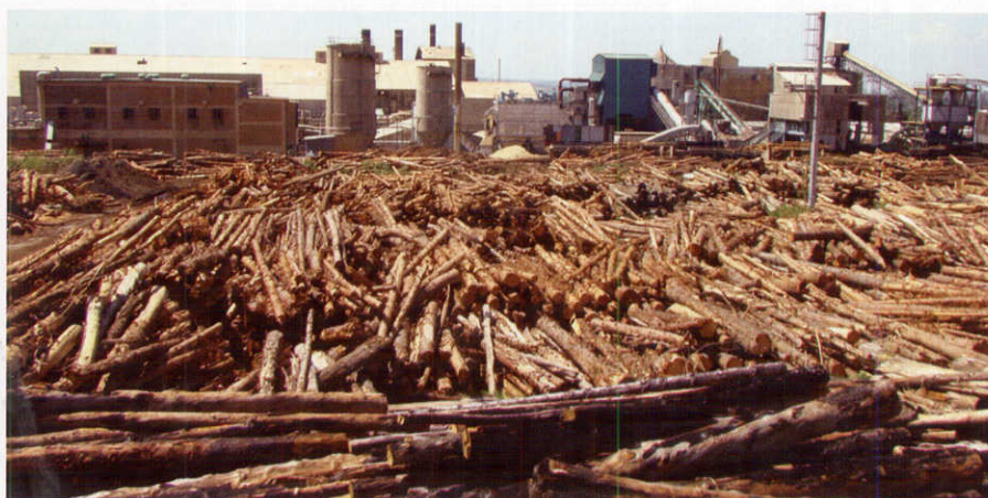
The log yard of Pan African Paper Mills in Webuye. Since this wood is for pulping for different types of paper, the quality of the logs (knots, straightness, etc) is not important. Note the scarred logs on the foreground, salvaged from a forest fire. (Photo: KFS)
