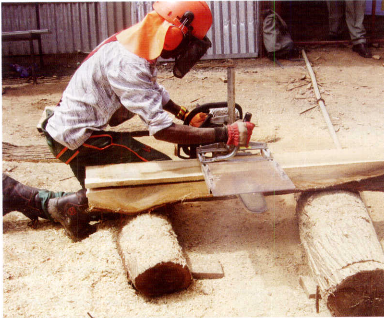
Framed chainsaw: A frame is attached to the chainsaw so that timber is sawn in a regular way, into planks of equal thickness. (Photo KEFRI)
