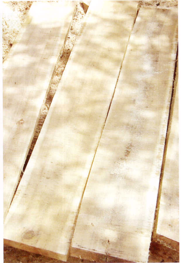
Framed chainsawn timber: This timber is produced by a framed chainsaw, and it is regular and smooth on the surface. (Photo KEFRI)
