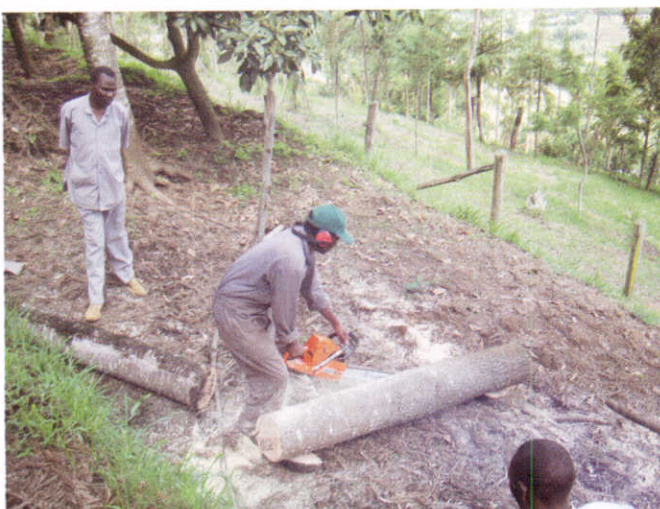
Freehand chain sawing is a common practice on farms. It is also called "splitting". (Photo: KEFRI)
