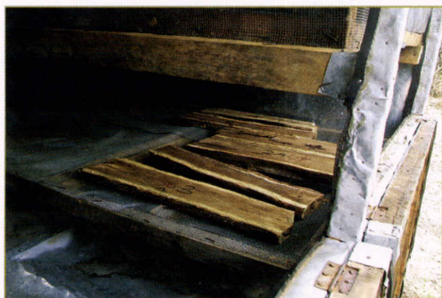
Samples drying in a solar kiln at Malindi
