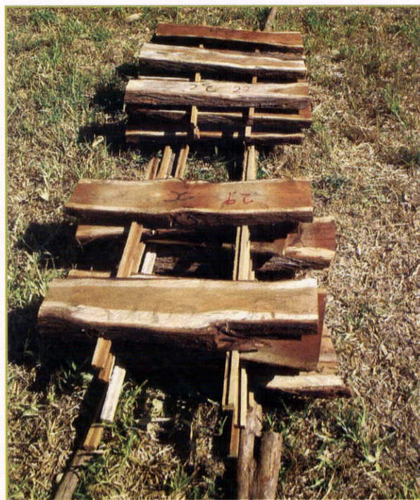
Prosopis samples undergoing the drying process at Malindi
