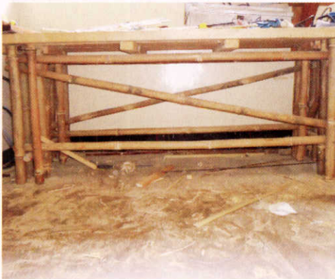
Work bench reinforced with diagonal braces.
