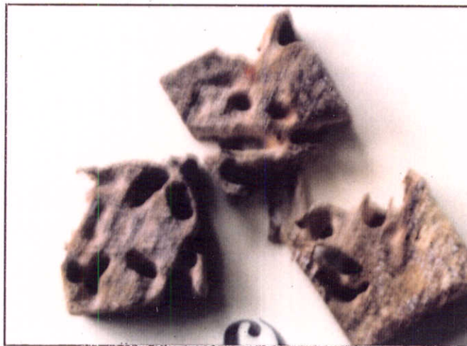
Plate 5.2: The extent of termite attack associated with the visual scores method of assessment of wood consumption
