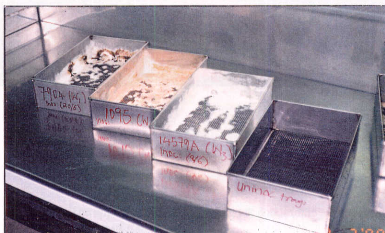
Plate 3.1: Fungal cultures at stage where blocks were introduced in decay chambers
