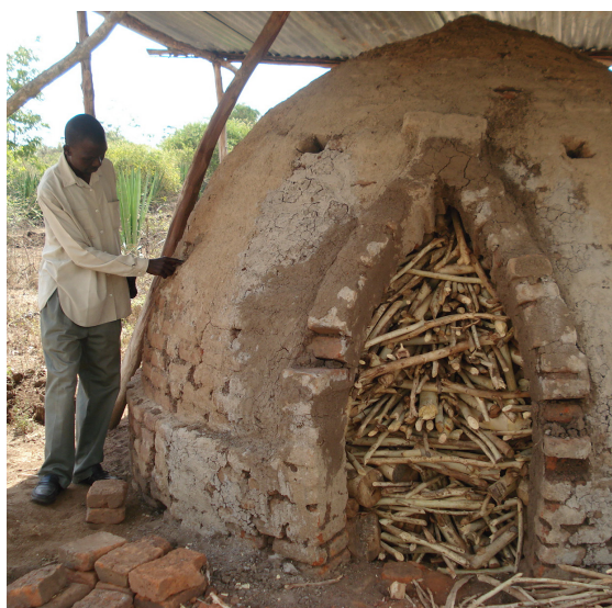
Figure 4.2: Wood arranged tightly inside a half orange kiln (Nellie Oduor, KEFRI)
