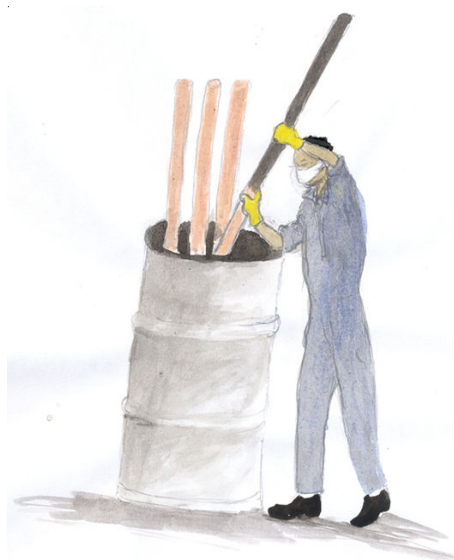
Figure 2: The debarked posts placed in a drum with preservative
