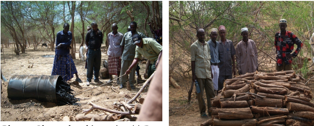
Plate 7: Charcoal making using (a) Drum kiln and (b) Earth kiln
