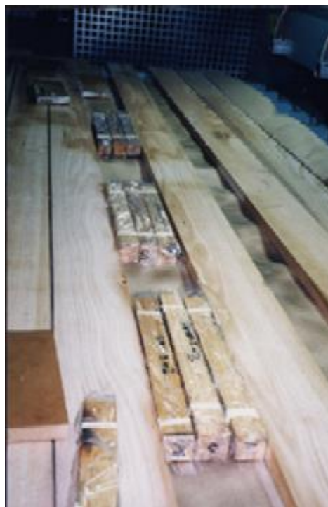
Fig. A2-1. Baioni press used for pressing of samples during the manufacture of Vintorg.
