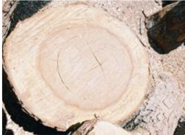
Fig. 2. End-grain of Neem log with eccentric pith from which radial shakes emanate.
