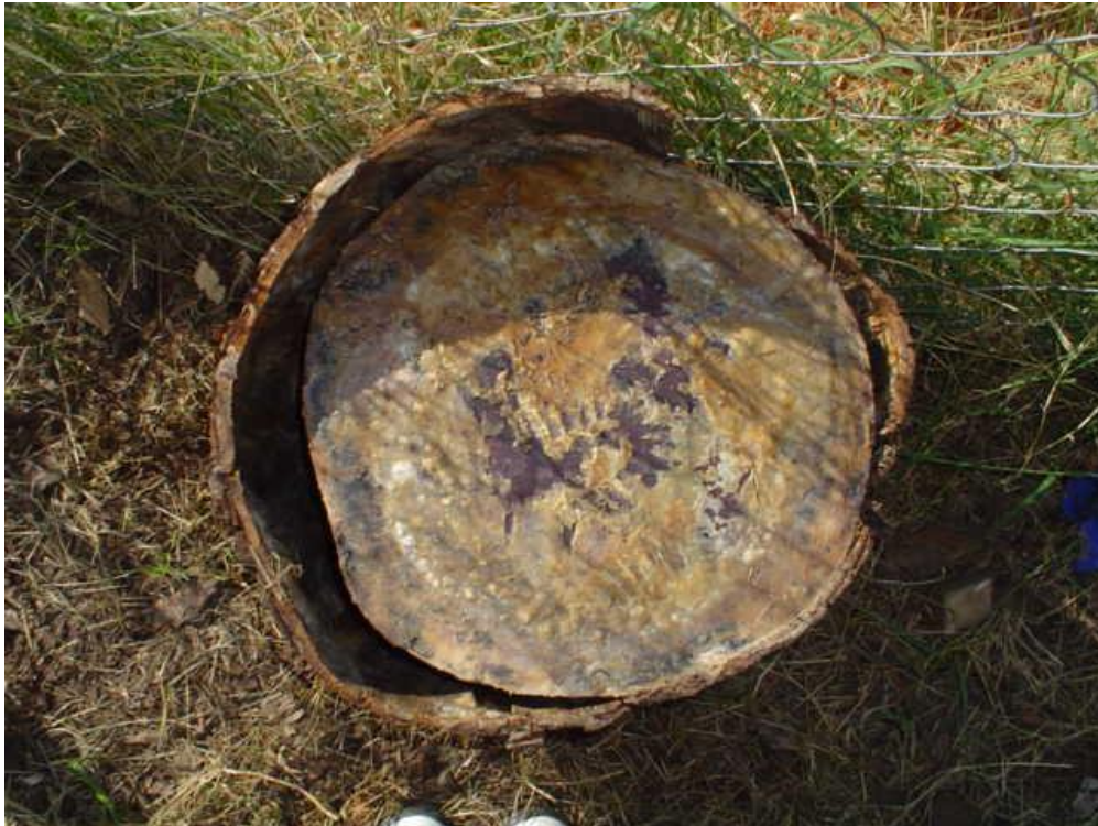
Fig. 2-7. Endsealed neem log put in the sun has bark peeling off.
