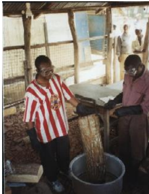
Fig. 4-1. Neem log being endsealed using paraffin wax.
