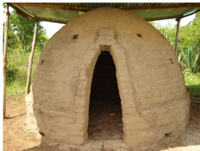
Plate 2: A half orange kiln in Madiany Division, Rarieda made of fired earth bricks
