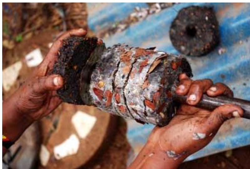
Plate 7: The circular hollow briquettes from the press laid out to dry before use
