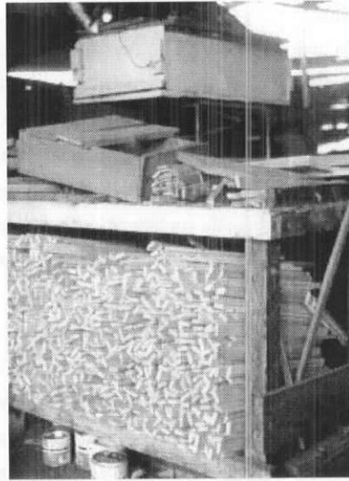
Fig. 4.2: Top bars that have been produced en masse to satisfy an order are seen here in storage. They are eventually distributed at random to different hives during final assembly of KTBH.
