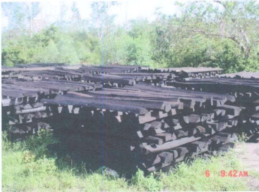
Plate 5: Treated posts well seasoned ready for the fencing.
