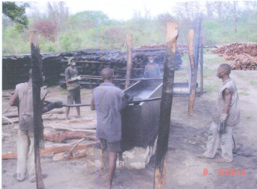
Plate 4: The team removing posts from boiling oil in the foreground already treated posts arranged to season in the middle ground while un- treated posts lie on the far right.
