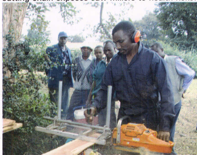
Timber sawing using a power saw
