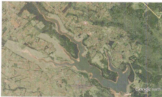
Sasumua dam on Sasumua stream, a tributary of Chania River, on the southern end of the Aberdare Range (on the right). Its designed storage capacity is 15.9 million m 3 , providing Nairobi with 12 per cent of its water supply.
