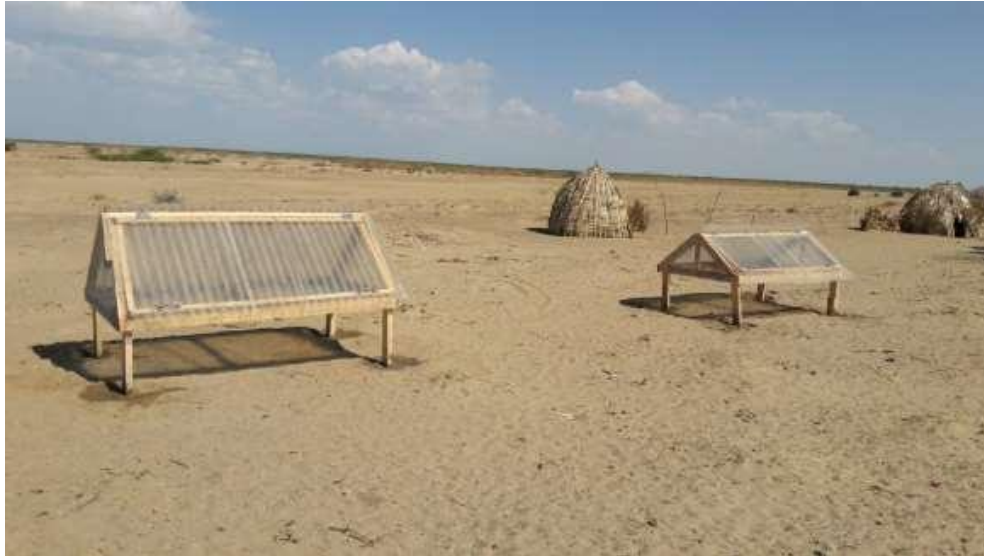
Figure 6: Solar driers installed using locally available materials and also community recommended sites near the beach.
