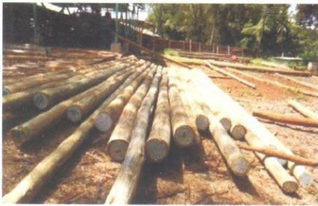
Plate 7: Power transmission poles
